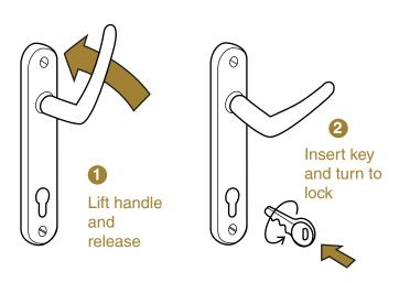
Allow the handle to return to the horizontal position. **To deadlock**, turn the key one full turn towards the edge of the door. This will secure all the bolts. In this condition the handle cannot be pushed down. Remove the key and place in a safe location.
